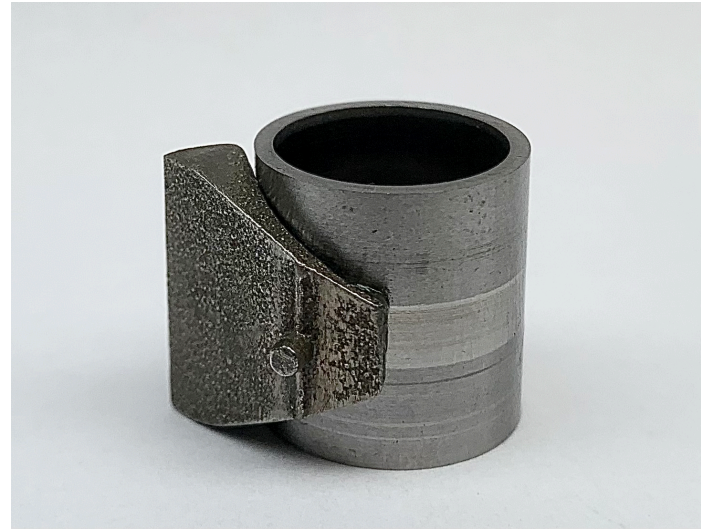
Fig. 7: A floating cup with a counterweight. The band on the cup is a result of the contact with the counterweight.
